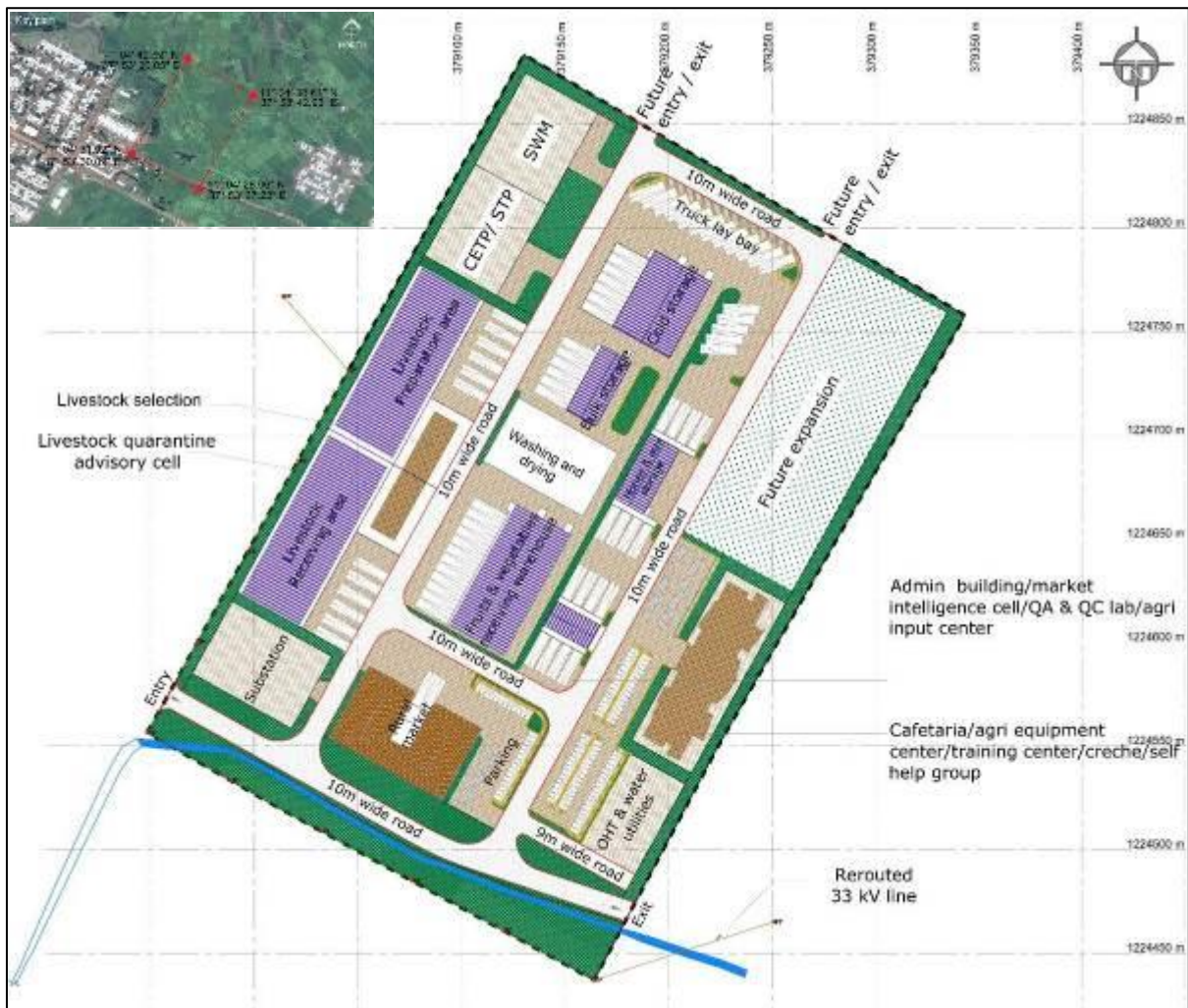
Figure 2-9: Site layout plan of the Motta RTC (Source: MACE master plan drawing)
