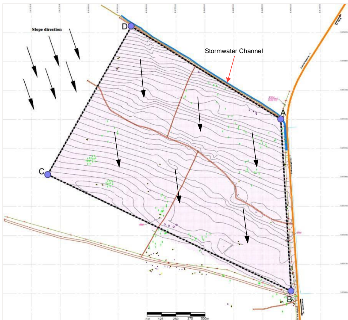
Figure 12 -1: Topography survey drawing of the IAIP site indicating predominate slope (Source: MACE)
