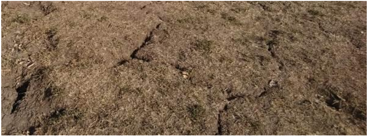
Figure 8-9: Photograph showing Arcadia / Vertisol surface cracking – SNNP IAIP site
