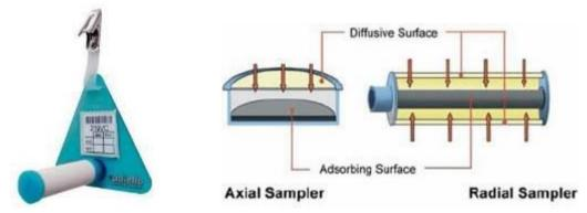
Figure 8-21: Diffusive and absorbing surfaces of a passive sampler SITE ASSESSMENT RESULTS
