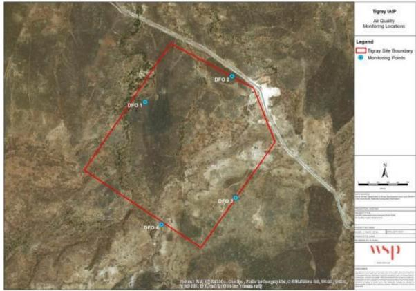
Figure 8-20: Dust fallout and passive monitoring locations at Tigray Baeker IAIP. Table 8-12: Coordinates of dust fallout and passive monitoring locations at Baeker IAIP.
